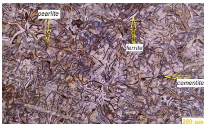
Figure 3. Microstructure of carburizer 91.57% (100X, Nital 3%).
