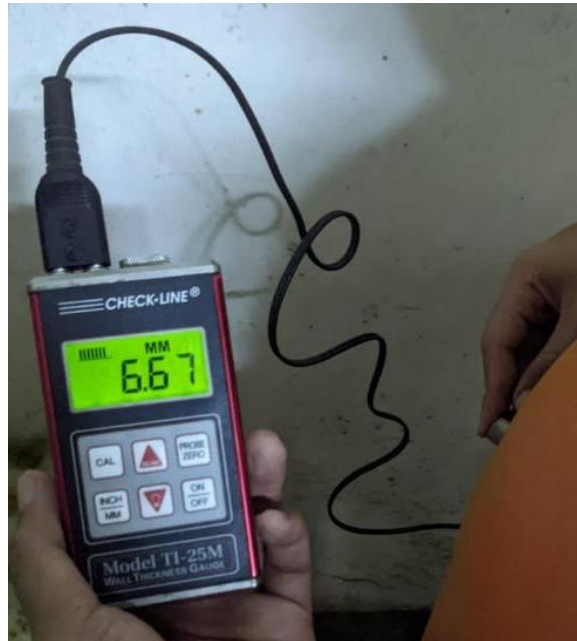
Figure 5. An example of measuring the actual thickness of a pressure vessel.
